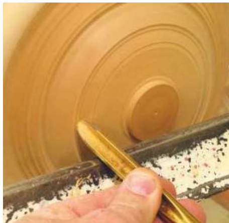
▲ Pic.11 Normally I like to do the final shaping of the bowl's exterior using the 6mm bowl gouge, but as I couldn't get the toolrest close enough, I required the strength of a bigger tool
